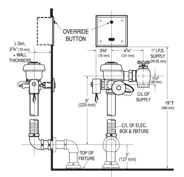
+ Position of Sensor Box can be raised or lowered 1" (25 mm) if in conflict with Handicap Grab Bars.
